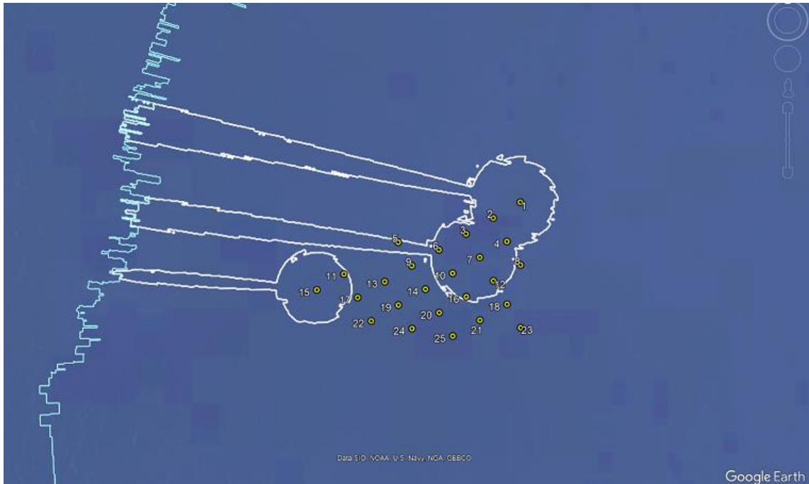
Figure 8 – UHF Tx: site C/I <23dB at 500ft
