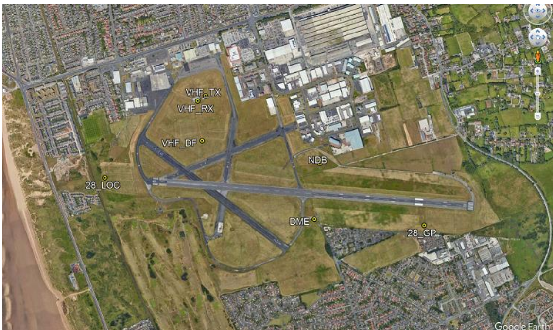
Figure 2 – On-airfield CNS equipment
