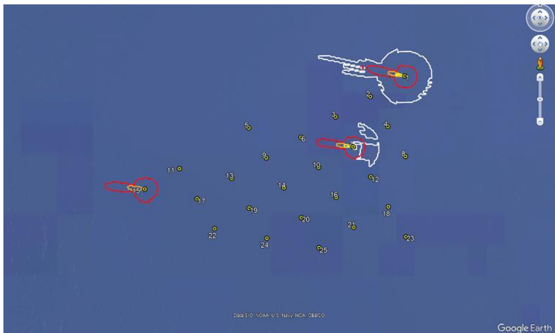
Figure 5 – VHF Tx site: C/I <23dB at 500ft – 4,000ft
