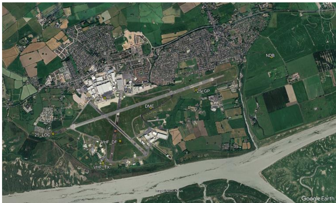
Figure 2 – On-airfield CNS equipment
