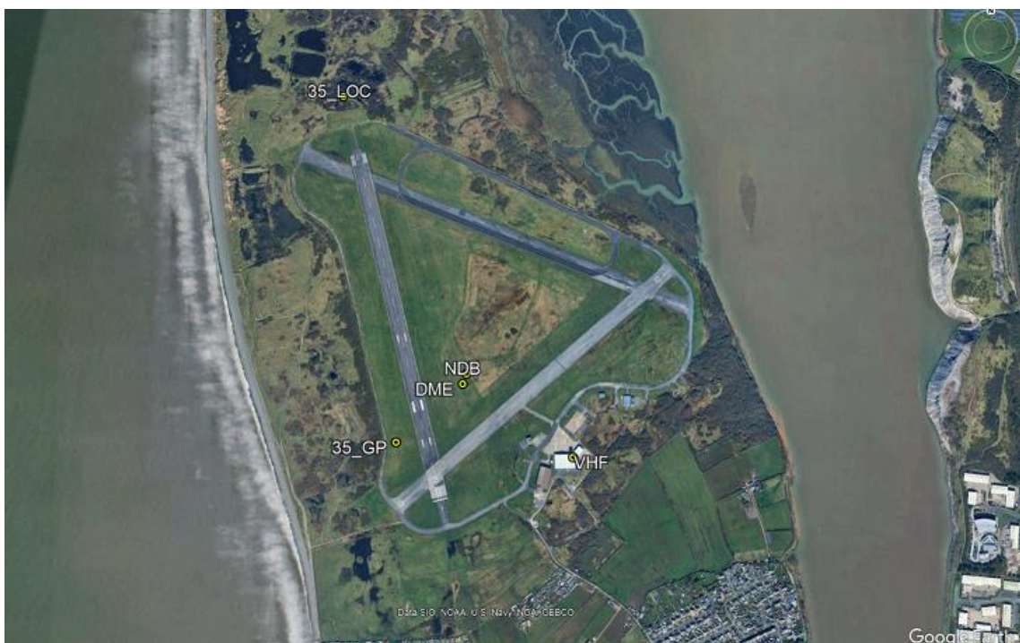
Figure 2 – On-airfield CNS equipment
