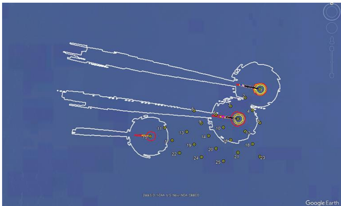
Figure 11 – UHF DF site: C/I <23dB at 500ft – 4,000ft
